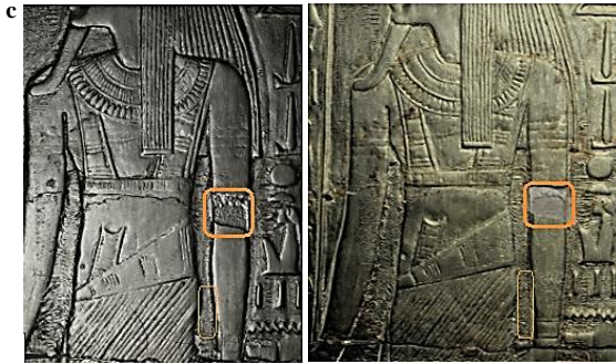
Figure (1) RTI images of gilding layer; a. creases in gilding layer, b. circular protruding dowel, buckling of gesso layer and brush strokes in gilding layer, c. brush strokes, creasing in the tight areas of the bas-relief and the layers of the rough and fine coat of the gesso layer in the missing part of the left elbow.
